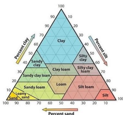
Figure 3. USDA diagram for soil textures
